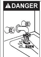
Water temperature over 125°F (52°C) can cause severe burns instantly resulting in severe injury or death.
